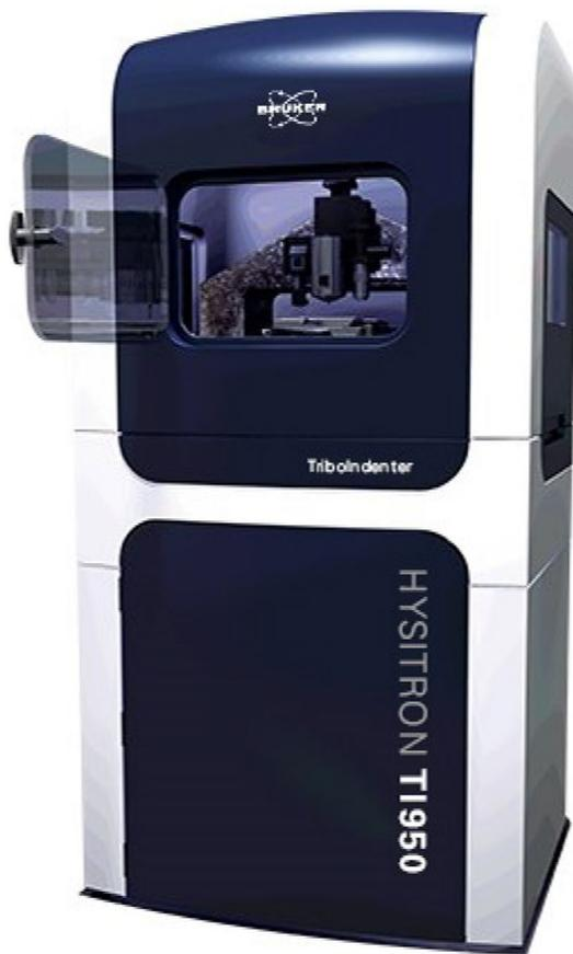
**Fig. 2** The Hysitron TI 950 indentation platform exploited to perform the indentations
